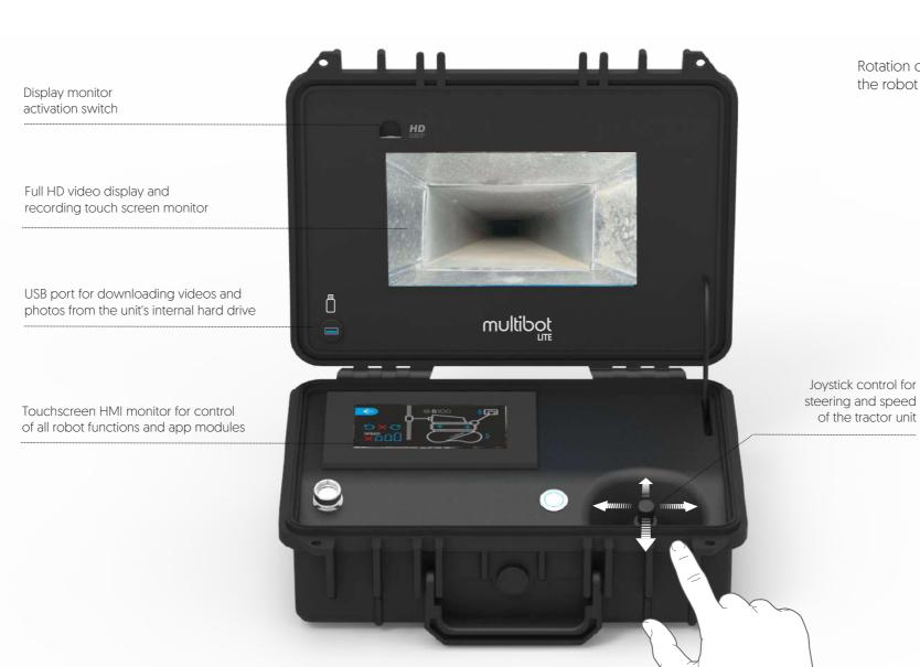
Rotation on 360° the robot shaft Speed-adjustable rotation, forward and reverse by joystick
